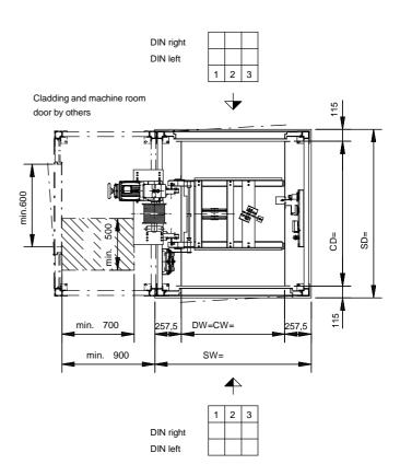
For an existing masonry or concrete shaft, smaller shaft dimensions are available on request!
