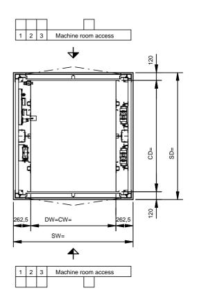
For an existing masonry or concrete shaft, smaller shaft dimensions are available on request!
