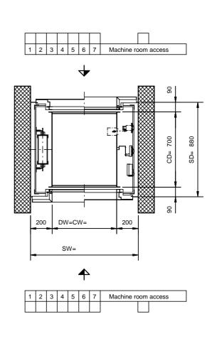
The shaft must be rectangular and perpendicular. Maximum admissible deviation from plumb is +20 mm -0 mm. All dimensions are minimum dimensions.
