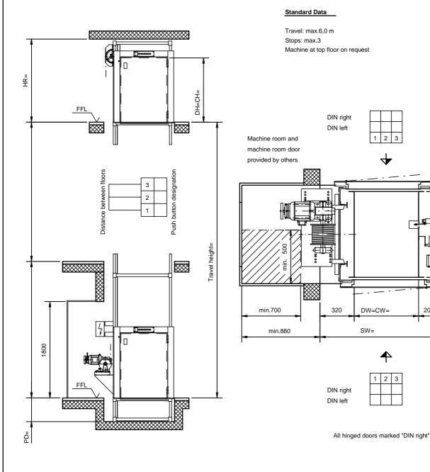
The shaft must be rectangular and perpendicular. Maximum admissible deviation from plumb is +20 mm -0 mm. All dimensions are minimum dimensions.
