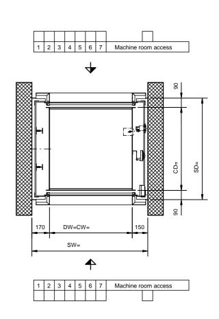
The shaft must be rectangular and perpendicular. Maximum admissible deviation from plumb is +20 mm -0 mm. All dimensions are minimum dimensions.
