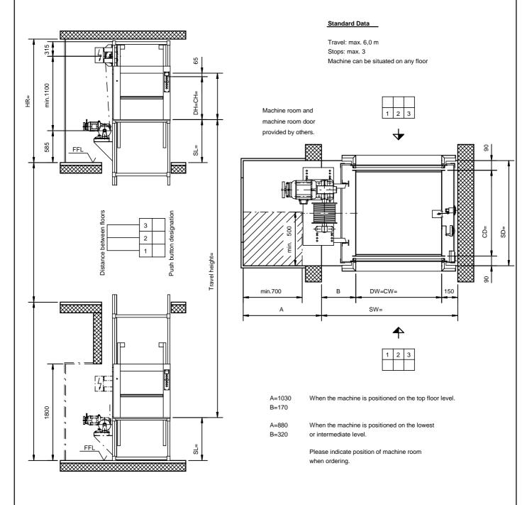
The shaft must be rectangular and perpendicular. Maximum admissible deviation
